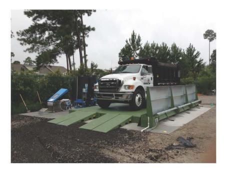
Flip screens on this 14' wide by 24' long Hydropad above ground steel containment wash rack are in the clean out position. Pull back the handle to flip the screen and clean out the collected grass and debris. Quick and easy screen maintenance. Return the flip screens to the operating position and shovel dewatered debris.
